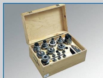
CODE 9459210 (CM4) CODE 9459212 (ISO 40): Cassetta completa di coni per frese a candela, per frese a spianare, mandrino portapinzette ø 4-20, testa barenatrice ø 70 con attacco CM4 a richiesta attacco ISO 40. Box containing taper shanks for end and face-mills, gripper-carrying spindle for 4-20 dia. mm drills, 70 dia. mm bo- ring head with MT4 taper, ISO 40 taper.
