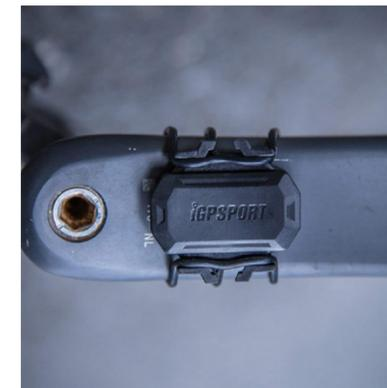
C) Finally, connect HOLOFIT to the cadence sensor using Bluetooth. It will automatically be visible in the pairing settings on HOLOFIT. Refer to step 9 for step-by-step instructions.
