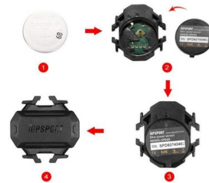
Open the back panel, put the battery in and close the back panel. The sensor will now start working.
