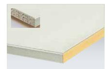
38mm particle board core with 1.2 mm galvanised steel cladding to surface, front and rear edges.
