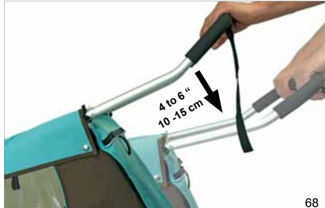
**Tip:** If you are not sure whether your Croozer Kid Plus is overloaded, you can perform this simple test **WITHOUT PASSENGERS**: Depress the handlebar of the loaded Stroller by about 4 to 6 inches to raise the Stroller wheel. Then carefully release the handlebar. If the Croozer Kid Plus immediately returns to its original standing position, then the Stroller is correctly loaded. If not, e.g. if the Croozer Kid Plus tips backwards, then the Stroller is overloaded and cannot be used.
