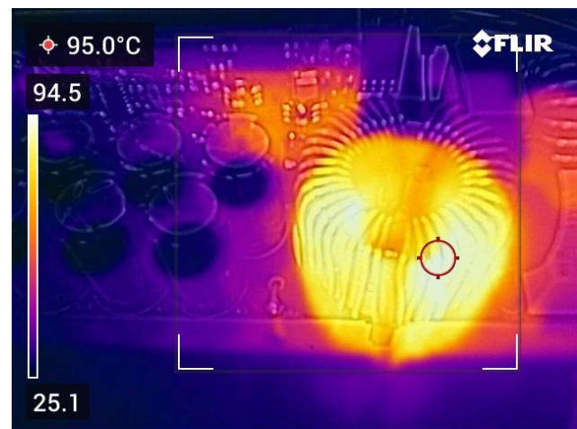
Figure 32 – PFC inductor temperature after 20 min at 115 V AC / 1.5 kW
