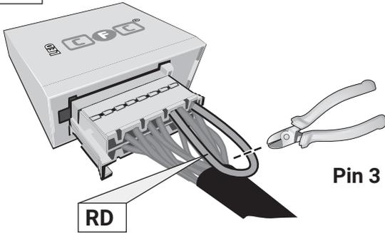
Pin 3 and Pin 2 disconnected
