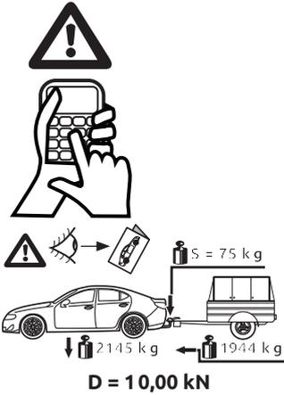
$$D = \frac{\text{MAX K G} \times \text{MAX K G}}{\text{MAX K G} + \text{MAX K G}} \times 0,0098 \leq 10,00 \text{ kN}$$
